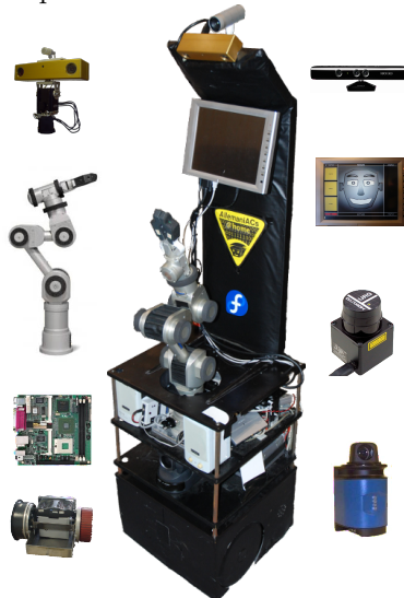
Fig. 1: Robot platform and its main components
