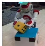
Fig. 1. Occurrence of an external fault while a robot places a die on a table. During the releasing action of the robot the orientation of the die causes the die to fall on the floor instead of staying on the table.
