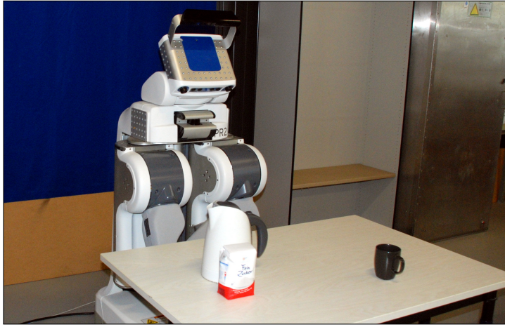
Figure 1. A PR2 robot looking at a table. From the current perspective, the sugar pack is occluded by the coffee pot and the handle of the mug is not visible, causing the robot to confuse it with a cup. From a different perspective, however, the robot would see the sugar pack and recognize the mug correctly. Hence, sensings from different perspectives are inconsistent.
