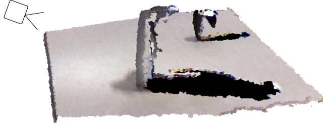
Figure 3. The point cloud as seen by the robot in Figure 1 and in the first perspective in Figure 2. The dark edge is the long edge of the table faced by the robot. Black color indicates shadow areas. Note that the sugar pack and mug handle are not visible.
