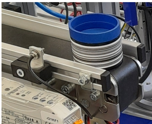
Figure 24: Image of a conveyor belt at the output side of an MPS with a laser mounted at its left and a workpiece on top.
