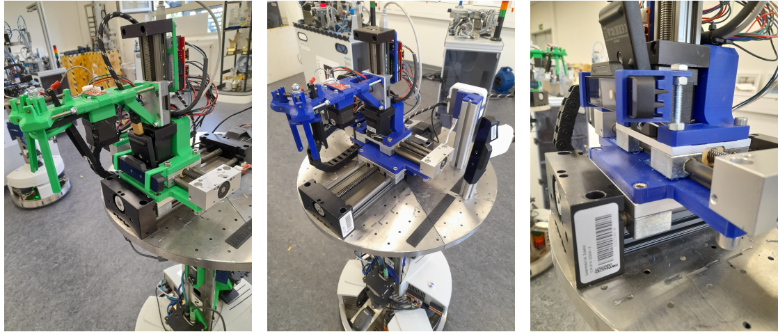
(a) Camera positioned at the gripper and used for the ICP approach. (b) Fixed camera with large distance between it and target object. (c) Camera positioned at the gripper with an offset to the position in (a).
