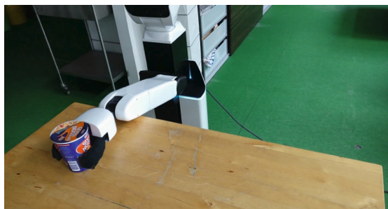
Figure 10: The robot successfully grasps a cup using whole body motion [25].
