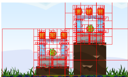
Figure 2: Quadtree of a scene, used to hierarchically structure the potential targets for simulation
